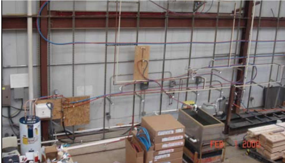
Figure 8.2 – Laboratory Test Set-up with Five Outlets, Hot Water Tank, and T&B System
